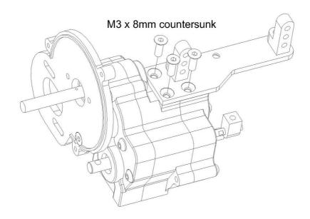
Now install the slipper clutch and spur gear the same way as on the stock Axial transmission.
